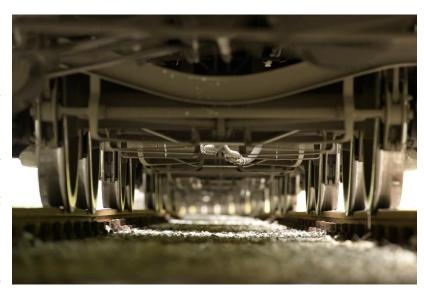
wagons with the new LL composite brake pads. The ban on loud freight wagons was introduced in Switzerland already in January, and the regulation will apply in Germany from mid-December. Retrofitting the wagons with quiet braking systems is particularly important for Rail Cargo Hungaria, as 80% of its transports are international.
