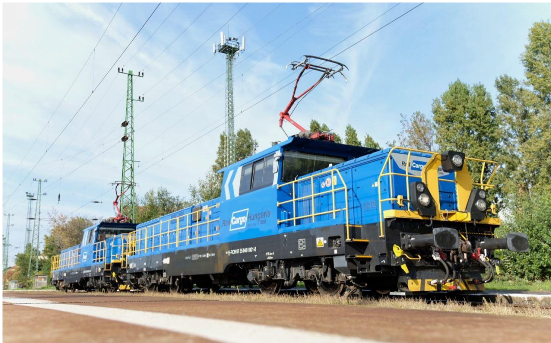
Electric hybrid shunting locomotives of Rail Cargo Hungaria
